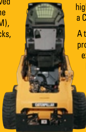
The C-Series cab tilts up and secures to allow convenient ground-level access to hydraulic pumps, motors, valves, lines and the hydraulic tank.
